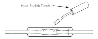
6. Properly installed, shrink tubing will be smooth and conform to the cable. Adhesive should be visible at each end of the shrink tubing.
