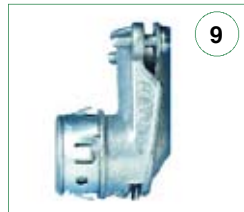
9 Size: 3/8": P/N E00-015-000 1/2": P/N E00-005-001 Type: Set Screw, Snap-in, 90° Material: Die Cast Insulated: No
